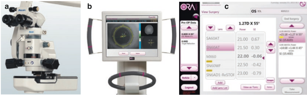
Figs. 45.3 ORA system™ (Alcon): (a) Aberrometer adjusted to the operating microscope. (b) Centration and alignment screen. (c) User interface
